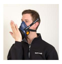
**NOTE!** If any leakage is detected, check the inahalation and exhalation valves, adjust the straps of head harness or switch to alternative size of the respirator. Repeat the fit check until there is no leakage.
